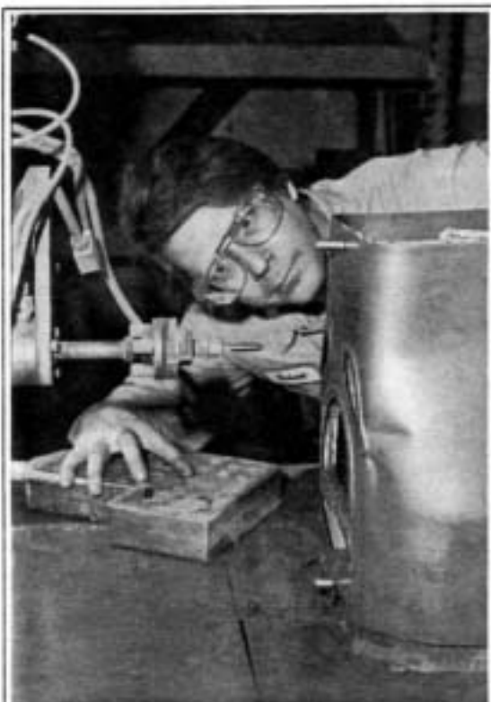
Flameco abrasive jet operator Robert Kirchmer times the set-up of the PASER II™ cutting head to produce military aircraft engine parts from stainless steel, titanium and other materials. Photo courtesy of Flow International Corp.
