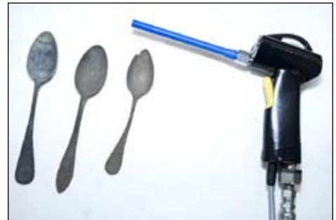
Three of the spoons cleaned with the Cold Jet i 3 MicroClean.
