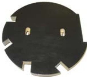
A steel gear cut from 3/4-inch steel plate.
