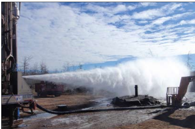
A borehole mining tool undergoing a surface test at a manganese borehole mining site near Emily, Minnesota.
