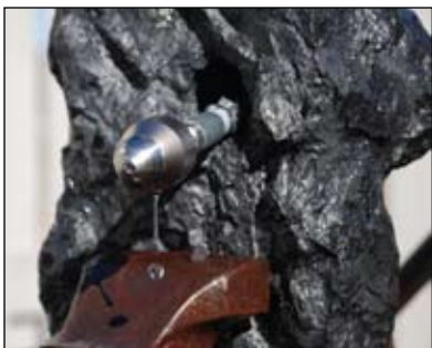
The Badger BA-L9 blasting through 6 inches of coke.
