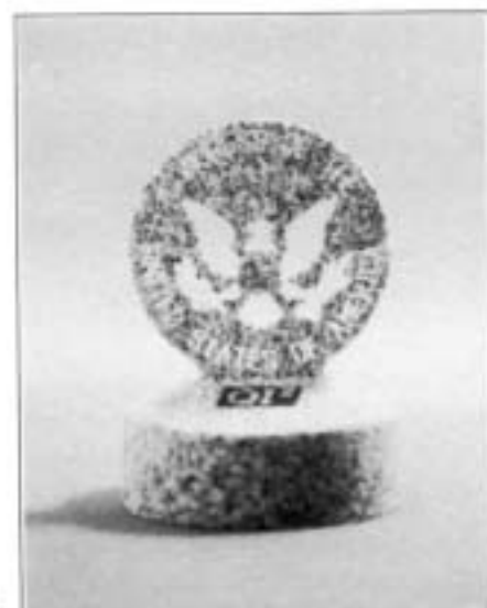
Abrasive water jet used to machine granite. Photograph courtesy of Quest Integrated, Inc., Kent, Washington
