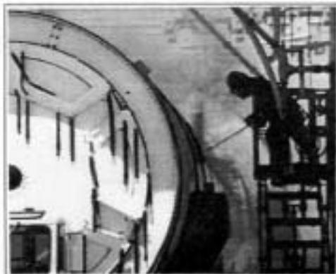
Manually Decoating A Space Shuttle Motor Segment
