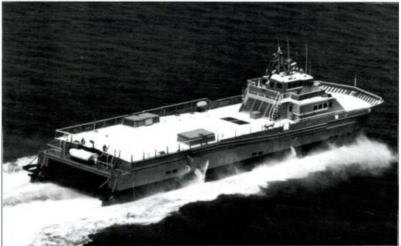
SES-200 with waterjet propulsion system. Photograph courtesy of U.S. Navy Domestic Technology Transfer Fact Sheet.
