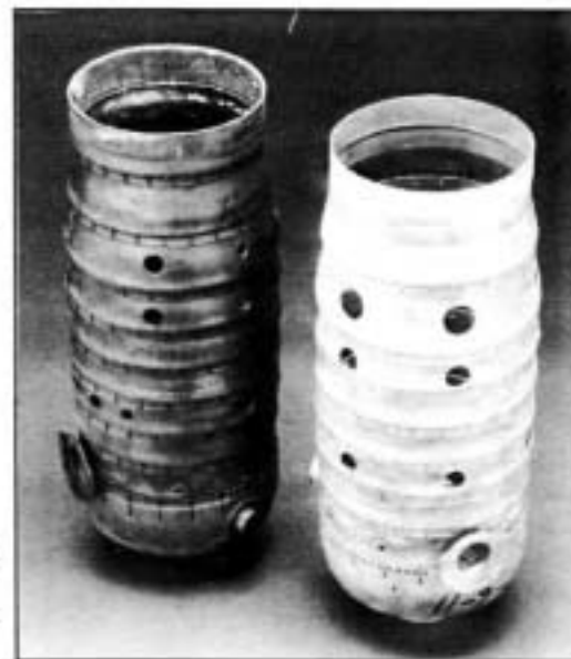
Two burner cans from a P&W JT8 engine. The left can has the ceramic coating in place. The ceramic coating and base coat have been removed from the right can with ultra high-pressure water.
