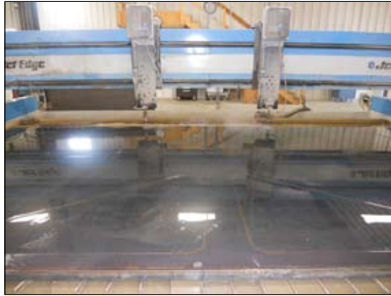
Mirror cutting a 12 ft. x 7 ft. 2-in. AR 500 plate.)
