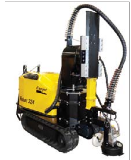
Conjet 324 Robot with optional rotor head.
