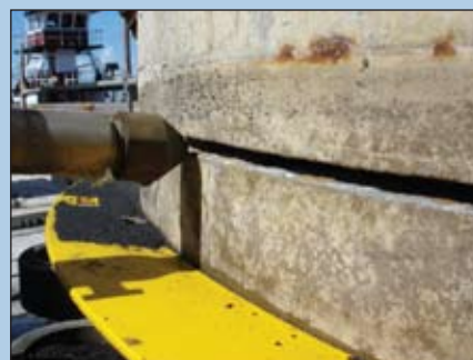
Proserv cuts steel pipe and removes two- to five-inch-thick concrete pipe coatings.
