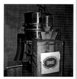
The Ward 24 will recycle abrasive and dry it, ready for reuse in about 3 minutes.
