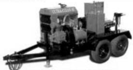
Model 4030D has a 44 hp diesel engine.
