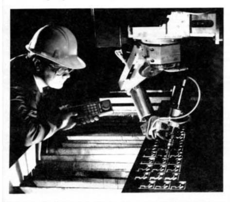
PASER IITM abrasive jet cutting systems manufactured by Flow International produce high-quality parts from tough-to-cut materials such as metal alloys, composites and laminates. Unlike other cutting processes, abrasive jets create no heated-affected zones and do no damage to even the most fragile parent materials. The process leaves a smooth, finished edge which minimizes or eliminates the need for additional machining operations. Photo courtesy of Flow International, Kent, Washington.
