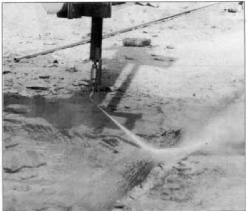
Oscillating water jet which cuts deep slots in hard rock.
