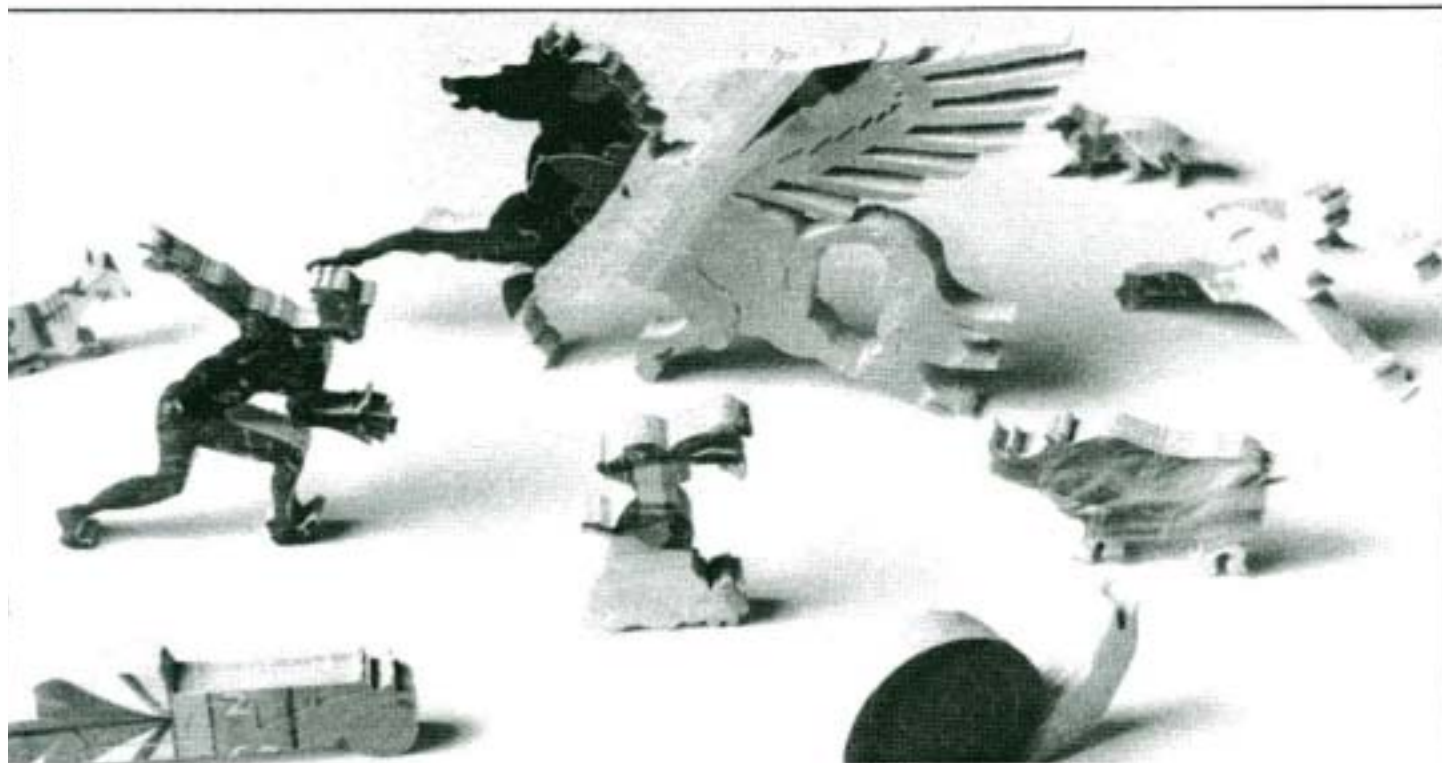
Parts of a puzzle cut by a water jet. Photo courtesy of J.C. Ayer & Co.
