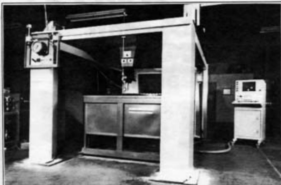
Ingersoll-Rand Waterjet Cutting Systems introduces the HS-1000, the first high-accuracy, X,Y and Z axis moving gantry system designed for cost-effective cutting in a wide variety of applications, including composites, plastic, foam, rubber, glass and metals.
