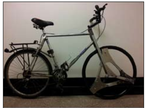
Hubless Bicycle. Called the hubless bicycle project, UBC students used the OMAX 2652 to create a non-spoke suspension system inside a bike rim.
