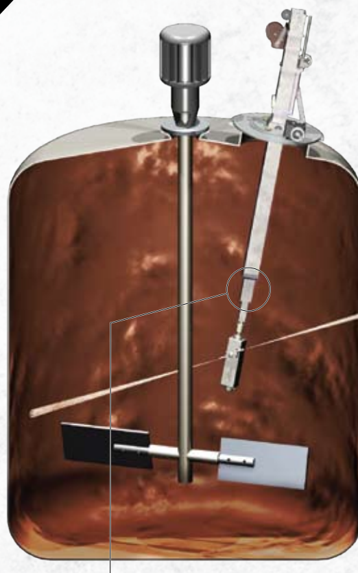
StoneAge® Teleboom shown here with Torus® tool. Telescoping arm can reach up to 19 feet. Teleboom and Torus® sold separately.
