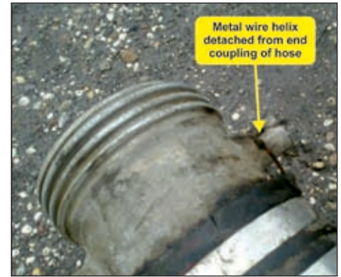
Figure 3 . An isolated coupling caused by a broken wire helix.
