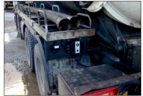
Figure 2: Example of a truck mounted (Earth-Rite® MGV) static ground verification system.
