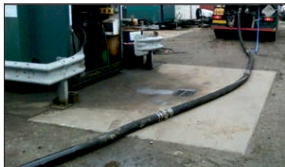
Figure 1. Four hose sections joined together in a vacuum truck operation with an OhmGuard® hose tester testing the first hose section (blue cable).
