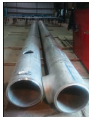
Midwest Mobile Waterjet of St. Paul, Minnesota used a Jet Edge-powered waterjet system to cut eight 10-inch holes into four 1.625-inch thick 24-inch diameter Inconel pipes for a high-temperature, high-pressure Louisiana refinery project.
