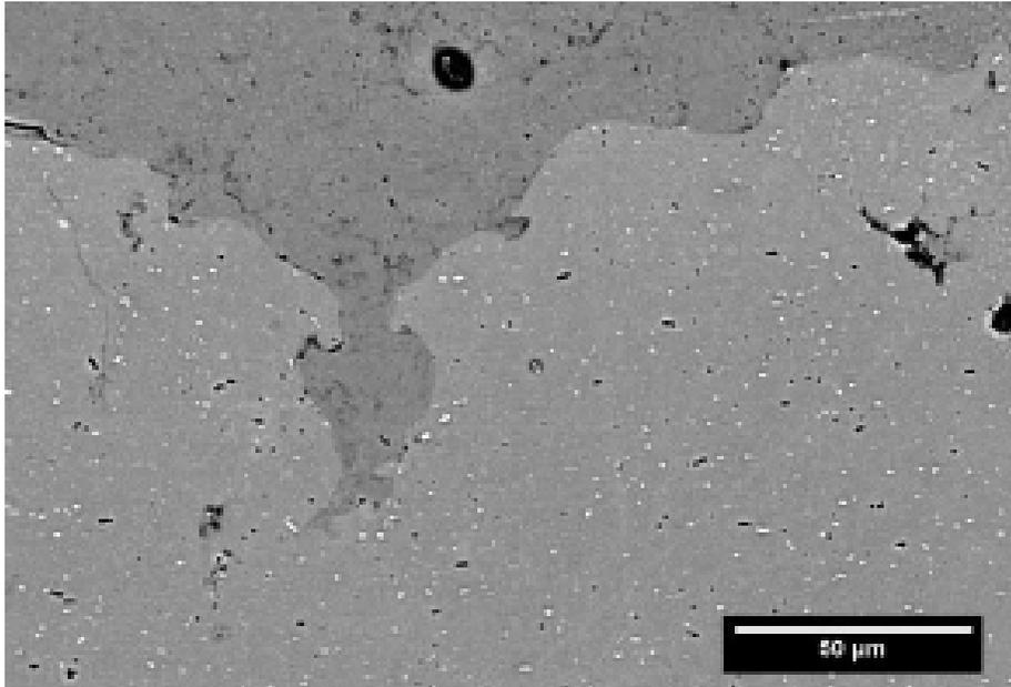
**Figure 15:** SEM image (500X) showing a cross sectional view of the coating and substrate interface. Note the interlocking effect offering strong mechanical anchoring.
