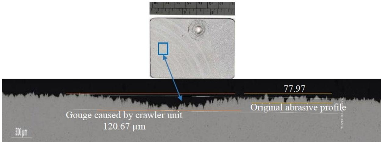
**Figure 61.** Metallographic images of an abrasive blasted Al 6082 coupon after UHPWJ for 20 seconds
