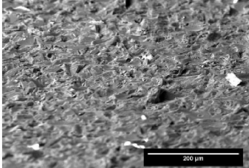
**Figure 13:** SEM image of grit blasted aluminum showing traces of alumina oxide grit embedment
