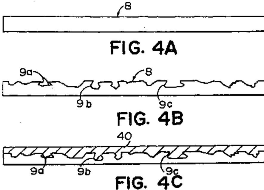
**Figure 10.** Depiction of cross section illustration the undercut for adhesion enhancement
