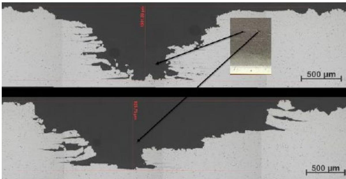
Figure 19 Metallographic cross-section images of two of the narrow gouges in the Al 5456 by a robotic crawler unit during the process of UHPWJ.
