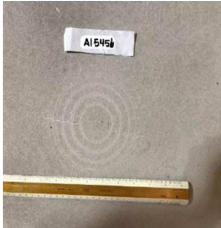
Figure 18 Combination of deep gouges in a linear direction and circular grooves seen into the Al 5456 plate. NSWCCD Figure
