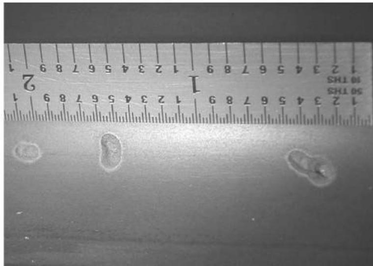
Damage at 250 MPa (36,000 psi), Time Periods of 10, 30 and 60 Seconds
