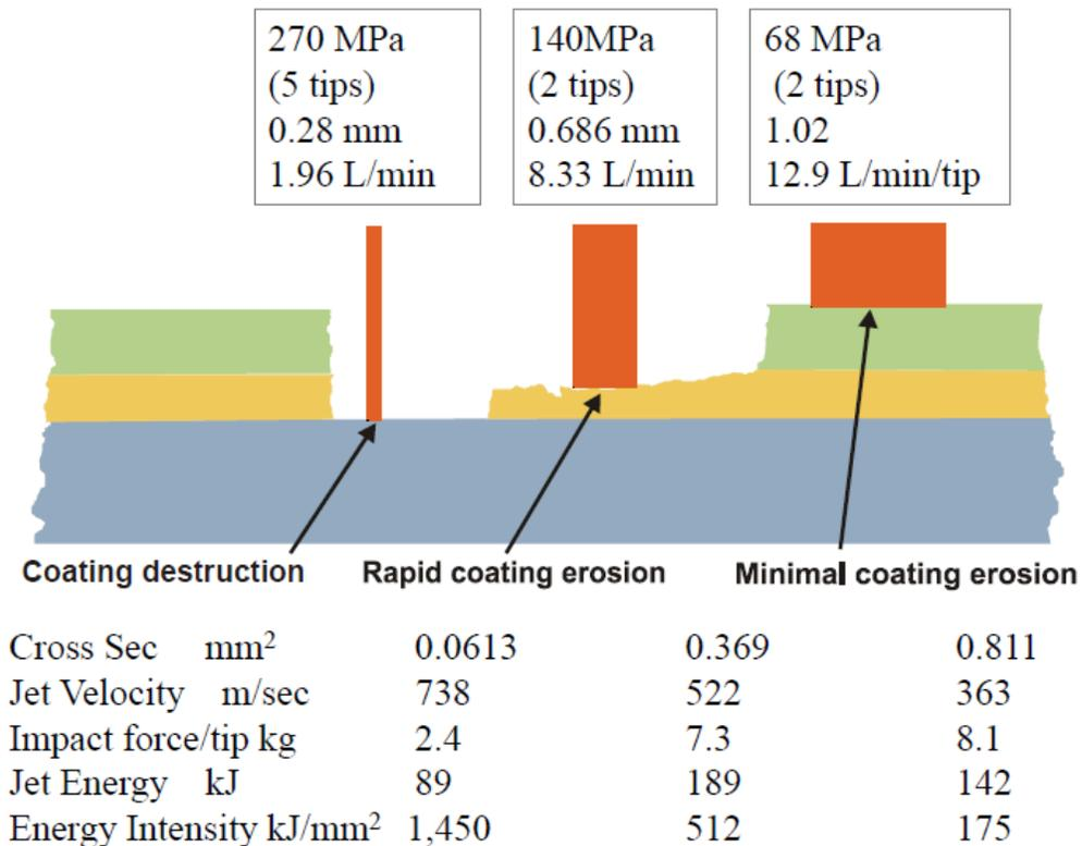
**Figure 1** Summary Graph of Pressure, flow, and Removal Reference 3
