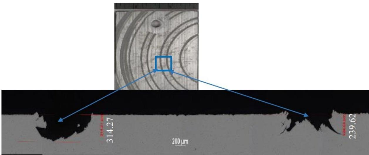
**Figure 68.** Metallographic image of a non-abrasive blasted mass loss coupon UHPWJ for 100 seconds in stationary position.
