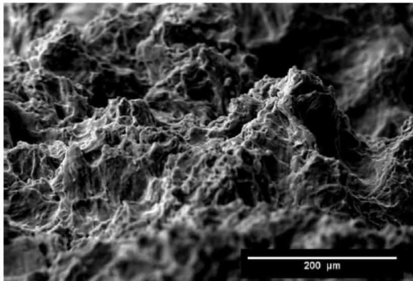
**Figure 14:** SEM Image (200x) showing PWJ roughened surface free from grit contamination.
