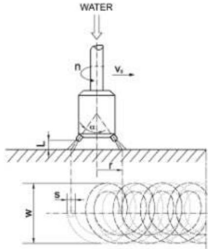
**Figure 5** Flat Surface Treatment Using Rotary Head Equipped with two water nozzles
