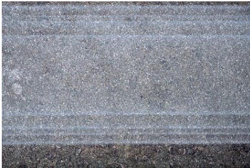
**Figure 4** Waterjet cleaning to WJ-1 of Grade D steel. The rotating head standoff was moved further in. Showing the linear groove of the nozzle.
