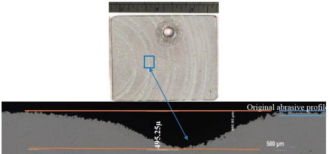
**Figure 71.** Metallographic image of an abrasive blasted Al 6082 coupon after UHPWJ for 120 seconds
