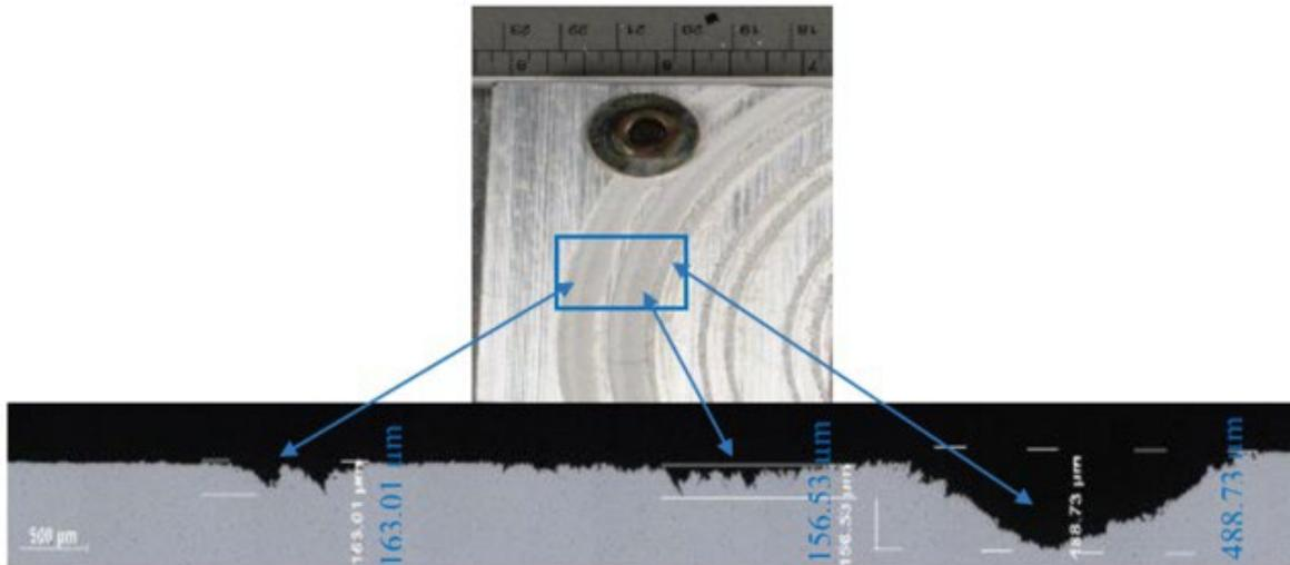
**Figure 70.** Metallographic image of a non-abrasive blasted Al 6082 coupon after UHPWJ for 120 seconds.
