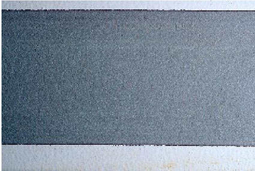
**Figure 3** Waterjet cleaning to WJ-1 revealing the abrasive blasted substrate. No measurable change in profile. The two layer coating system in white topcoat, red primer.
