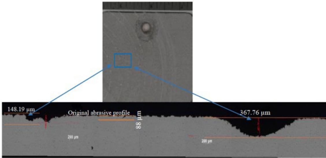
**Figure 69.** Metallographic image of an abrasive blasted coupon after UHPWJ for 100 seconds.
