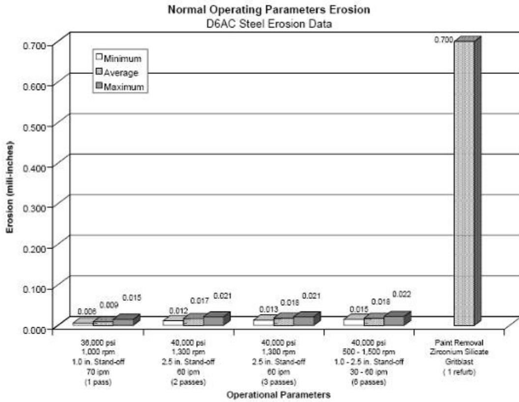
Figure 1. Waterjet Erosion versus Gritblast Erosion
