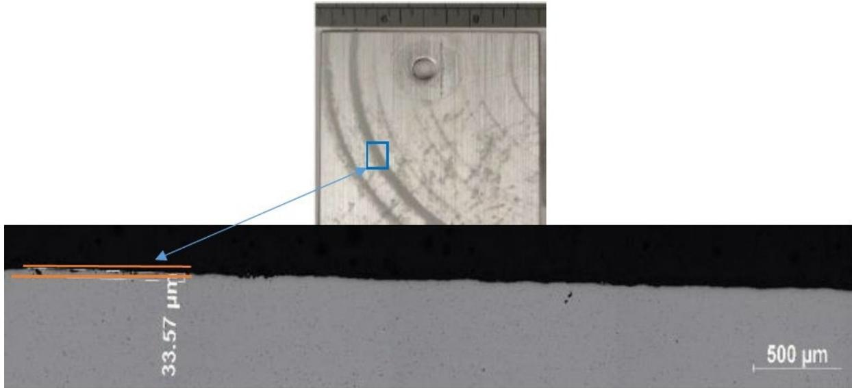
**Figure 58.** Metallographic image of a non-abrasive blasted Al 6082 coupon after UHPWJ for 10 seconds
