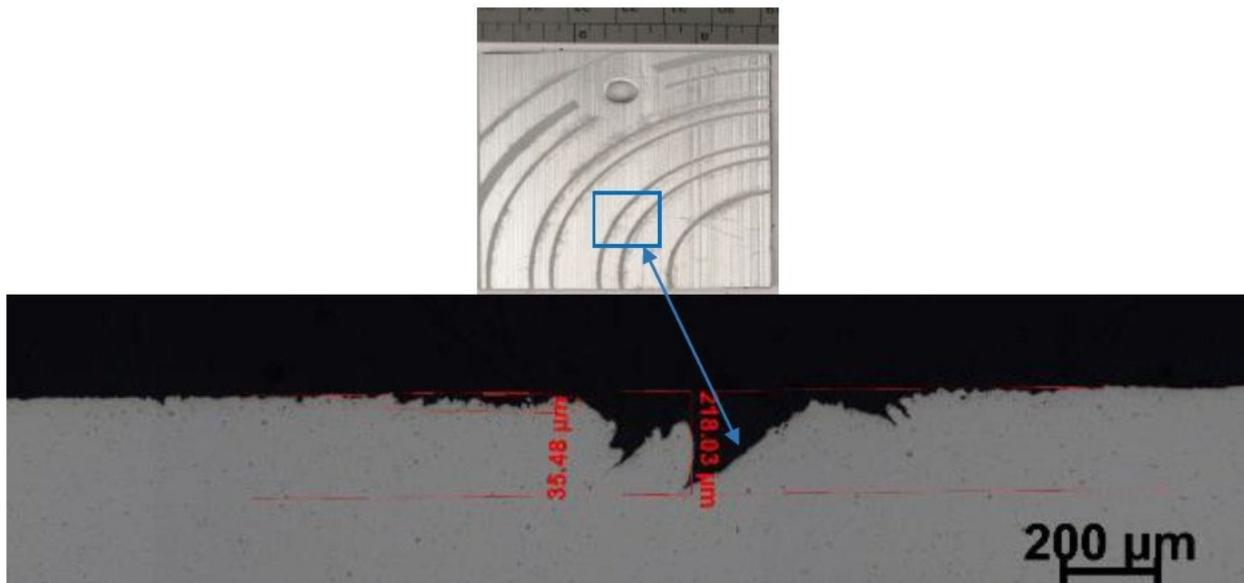
**Figure 60.** Metallographic image of a non-abrasive blasted Al 6082 coupon after UHPWJ for 20 seconds
