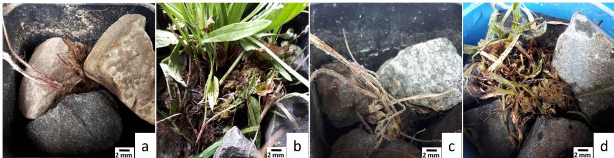
Figure 9. Run 8 and 9 (SOD = 200 mm, m_A = 200 g/min, \beta = 45 deg). a+b: p = 150 MPa (a: herb-Robert, b: ribwort plantain), c+d: p = 75 MPa (a: herb-Robert, b: ribwort plantain).
