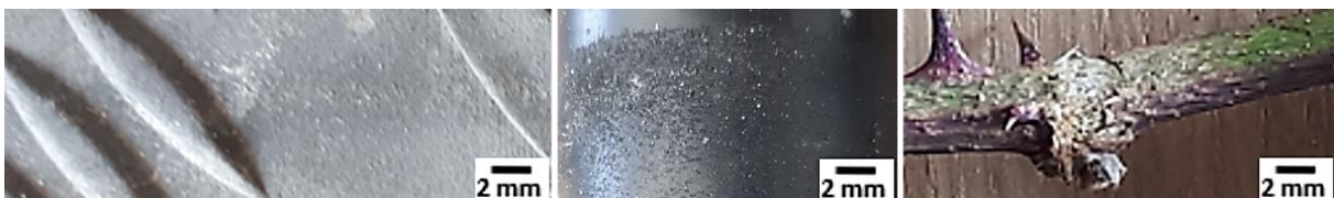
Figure 6. Results of AWJ (abrasive, \beta = 90 deg) at p = 150 MPa and SOD = 300 mm. Left: cover, middle: signal cable, right: blackberry vine.
