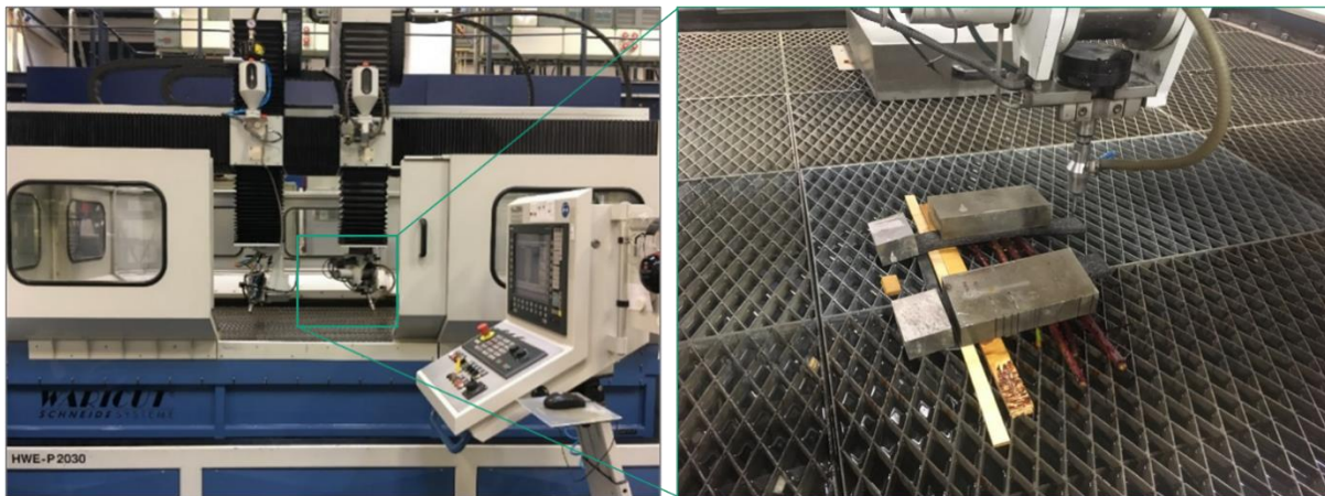
Figure 1. Waterjet machine and arrangement of the specimen.
