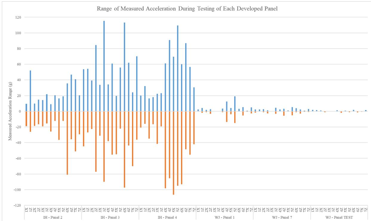
Figure 6. Range of measured acceleration during testing of each developed panel
