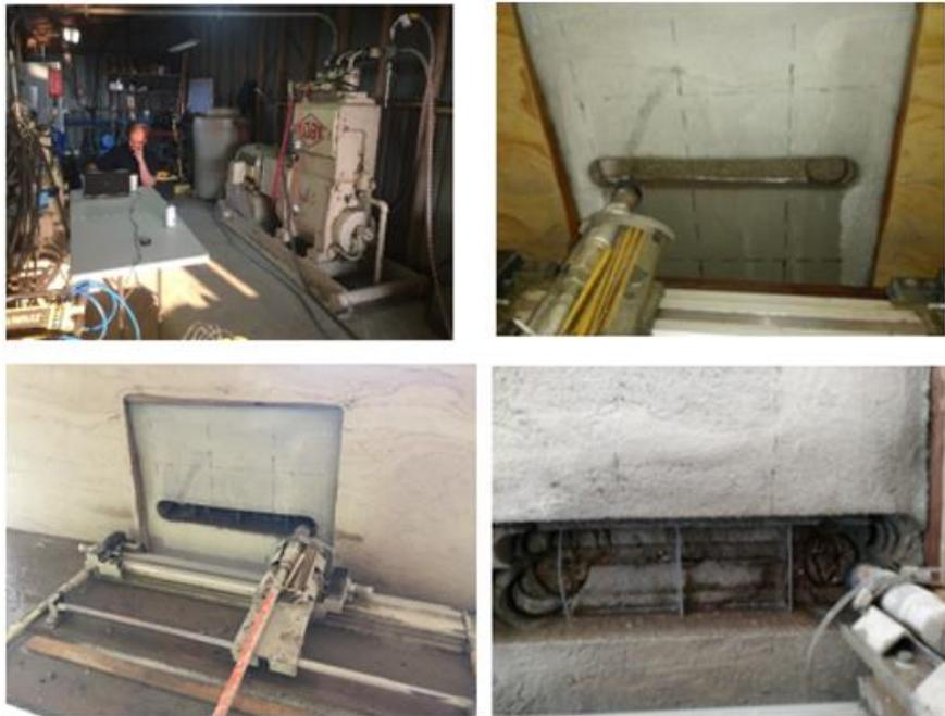
Figure 4. Waterjet excavation – Laboratory set-up (upper left) start of slot in panel (upper right) kerf in panel (bottom left) close-up of kerf in panel (bottom right)
