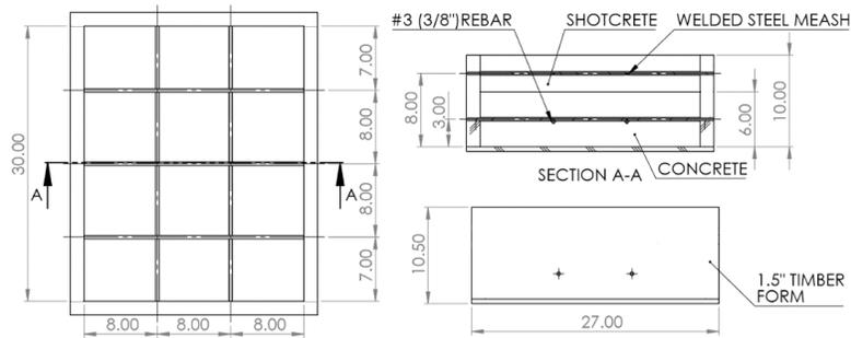
Figure 1. Composite panel dimensions (shown in inches)
