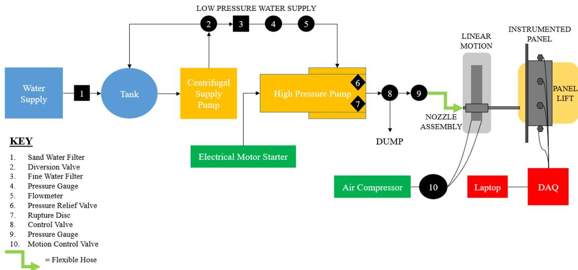
Figure 3. Waterjet instrumentation and cutting setup
