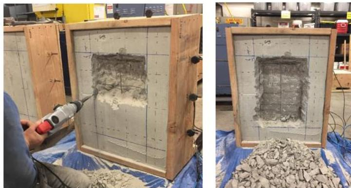
Figure 2. Process of mechanical excavation using impact hammer
