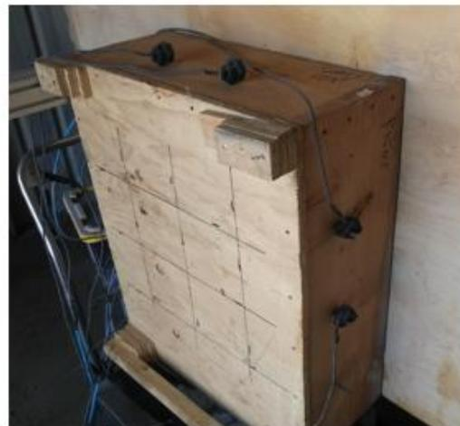
Figure 5. Accelerometer locations (left) accelerometers on actual panel (right)
