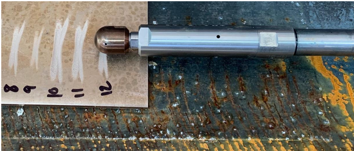
Self-Rotary Tube Nozzle Assembly Test Arrangement and Results in Copper Nickel Figure 2.
