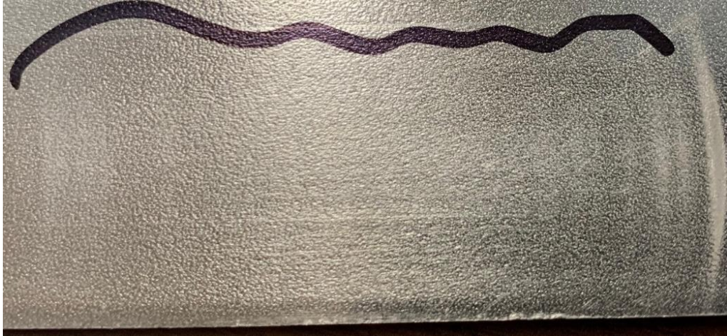
The Result of 50 Passes with Rotating Head at 228 MPa (33,000 psi) in Monel 400; Note Damage at End of Travel Range Where Pause of Direction Change Occurs Figure 17.
