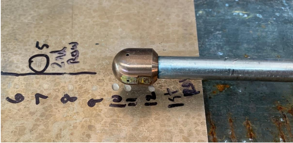
Non-Rotary Head Test Arrangement Shown with Copper Nickel 90/10 Sheet Figure 1.
