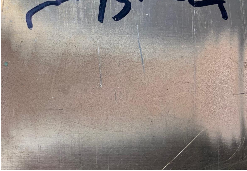
The Result of 100 Passes with Rotating Head at 103 MPa (15,000 psi) in Copper 110 Plate Figure 15.
