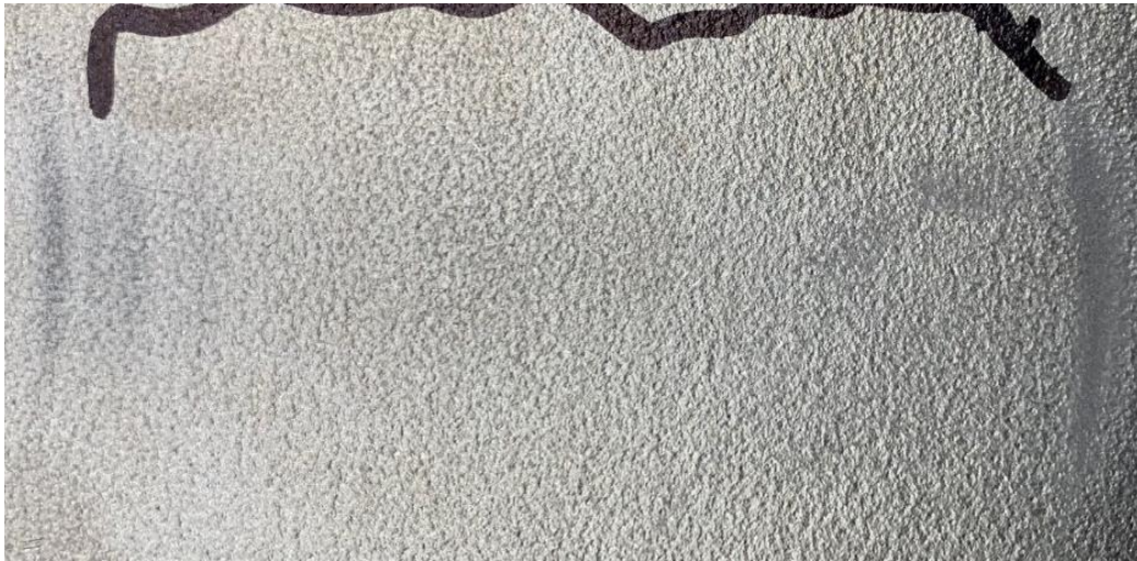
The Result of 50 Passes with Rotating Head at 228 MPa (33,000 psi) in Titanium Figure 18.
