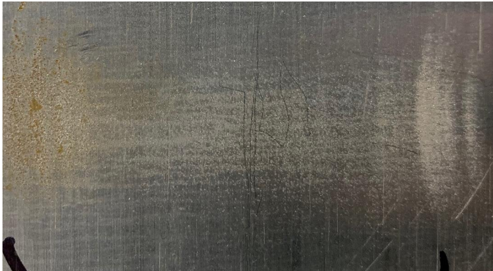
The Result of 50 Passes with Rotating Head at 228 MPa (33,000 psi) in 1018 CDF Plate Figure 16.
