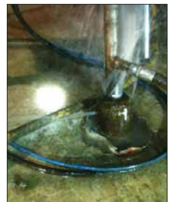
Jet cutting using polymer enhanced circulation aids in carrying returns to the surface.
