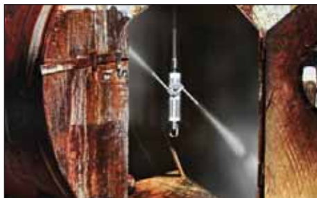
Jetstream's hands-free waterblasting solutions cover a variety of applications, including cleaning tanks, reactors and other large vessels.
