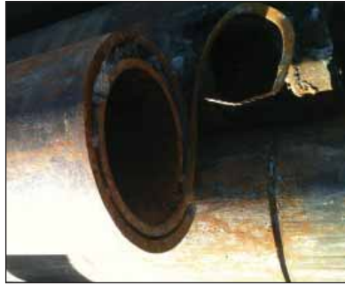
The hydraulic cylinders on the drill supporting the cutting head bled down while cutting causing this spiral effect.
