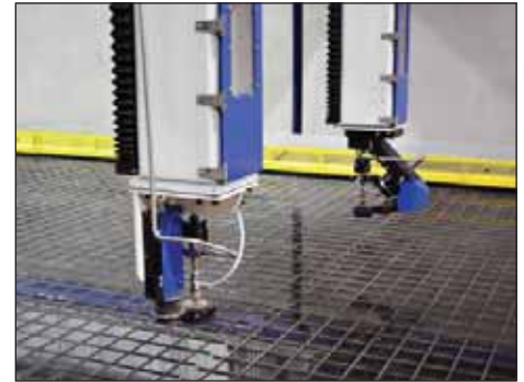
The GX-4816-5 large-scale waterjet features dual cutting heads with five feet of Z-travel and both 2D and 5-Axis capabilities.
