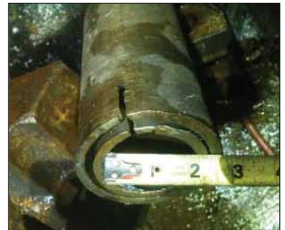
Very small casing sever and slot cut, 300 feet deep.
