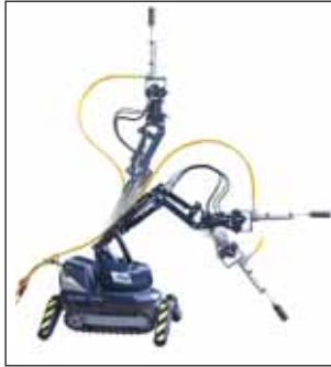
Versatile: The Woma Jetty - here with short lance support, suitable for working in areas where hand-held water tools cannot be used.
