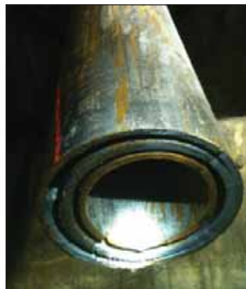
Three layers of casing cut at 300 feet deep recovered after over-coring.
