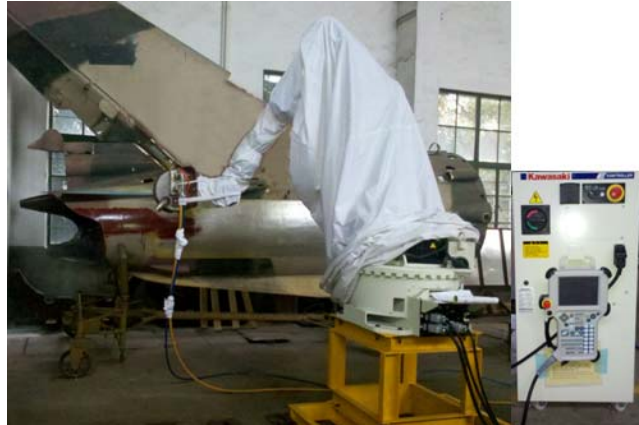
Figure 7. Six axes robot operating in airplane paint removal site Table1 Paint removal test
