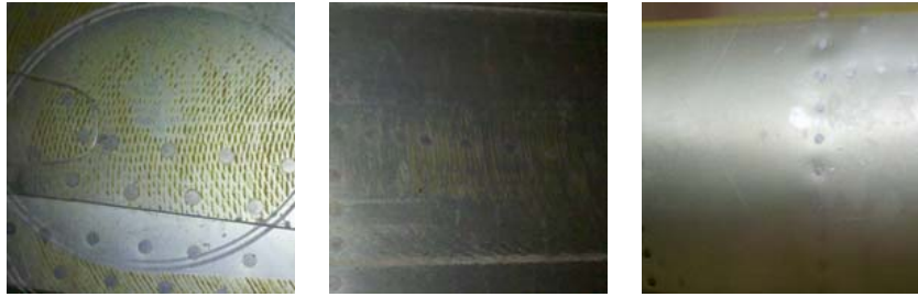
Figure 8a. Paint removal effect under 2.4m/min and different pressure
