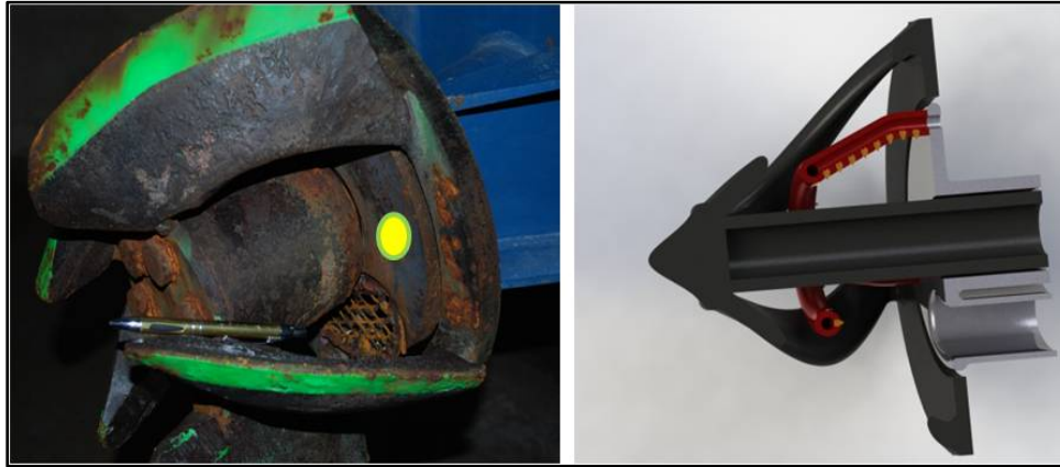
Figure 17. Location and Sketch of Waterjet Testing Apparatus
