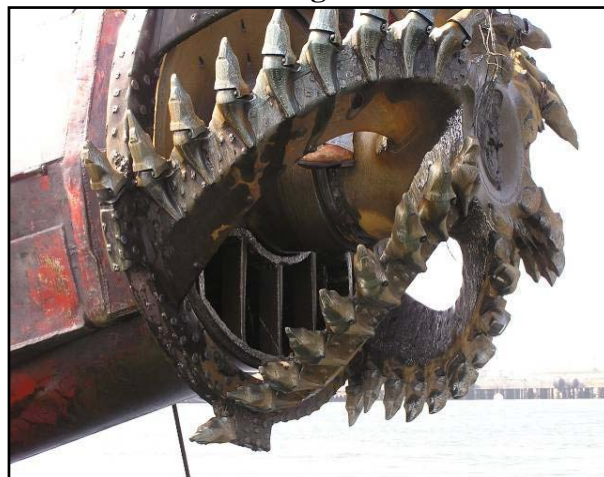
Figure 10. Rotary Cutter Showing Suction Inlet 12
