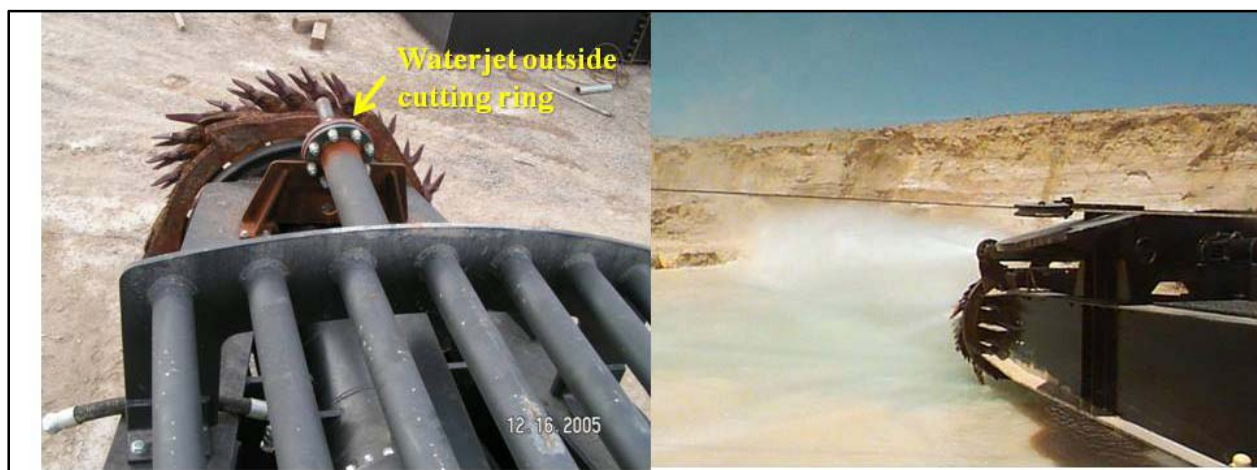
Figure 12 Dredge Supply Company's Waterjet System with a Cutter Head
