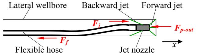
**Figure 3.** Force analysis of drilling system
