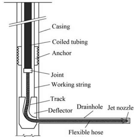
**Figure 1.** Schematic of radial drilling downhole system
