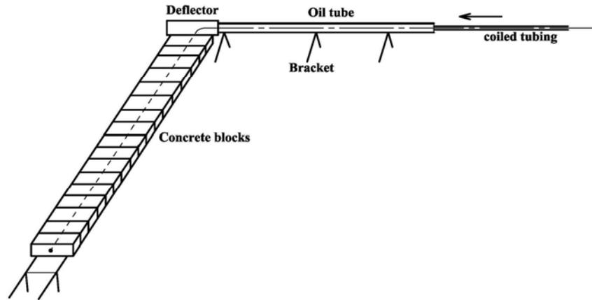
**Figure 13.** Schematic of ground test of hydra-jet radial drilling
