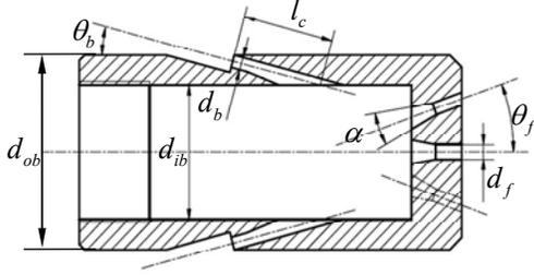
**Figure 2.** Structure diagram of jet nozzle
