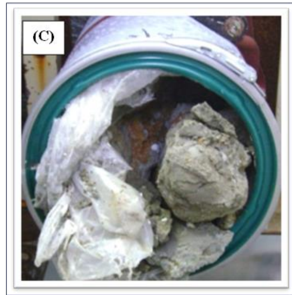
Fig. 7. Photograph showing the cutting of the lid with the FPWJ, exposing the concrete in the pail.
