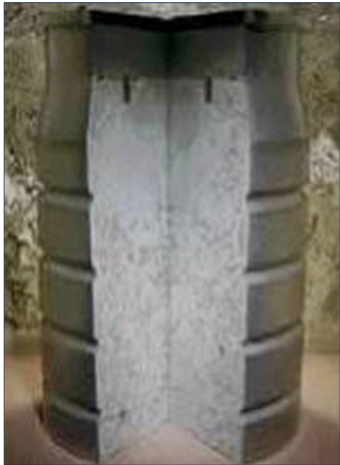
Fig. 1. A typical steel drum containing concrete mixed with the radioactive waste materials (Ref. 30).
