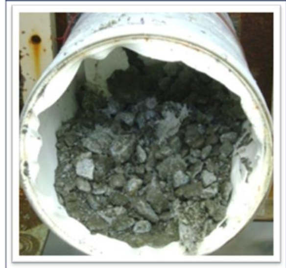
Fig. 9. Fragmenting the concrete within the pail with the FPWJ using the configuration as indicated in (A) and in (B).
