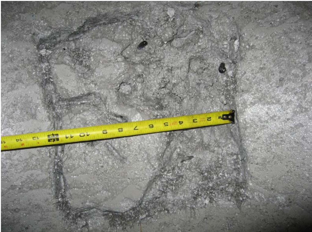
Results of Manual Chipping in Type 1 Refractory, 1 Hour Duration Figure 1.
