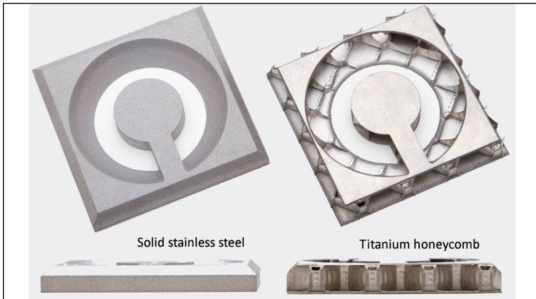
Figure 18. OMAX logos with bevel edges cut with A-Jet
