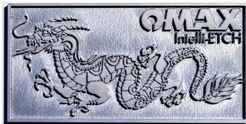
Figure 6. AWJ etching on an aluminum plate (Webers et al., 2010)
