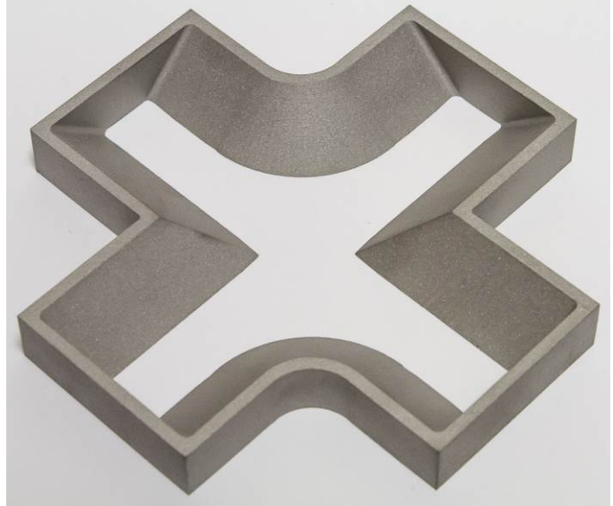
Figure 21. Software controlled bevel cut
