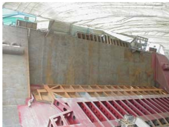
Figure 3 Rust Bloom USS Boxer Notice: Difference in amount between Vertical Sides and Sloping Girders
